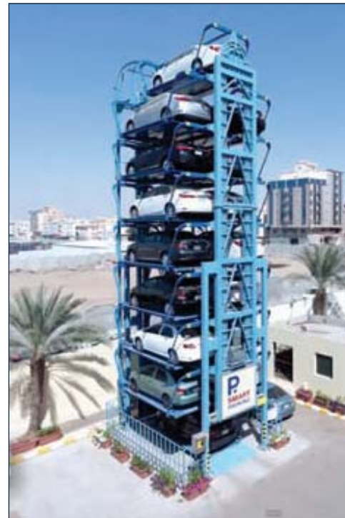
16 car parking lots by a unit of SM16L, Toyota car maintenance shop, Jeddah, Saudi Arabia
